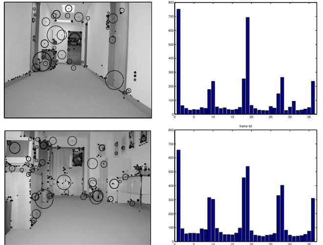
Fig. 1. Locations  $l5$  (top) and  $l3$  (bottom) of the 4<sup>th</sup> floor, detected scale invariant features and global gradient orientation histograms (right). The circle center represents the keypoint’s location and the radius the keypoint’s scale.
