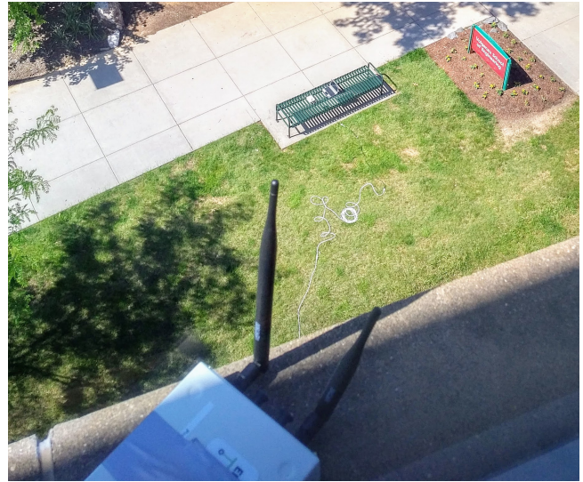
Figure 12: Test area used in for elevation tests. The receiver is placed on the ground and the sender is elevated.
