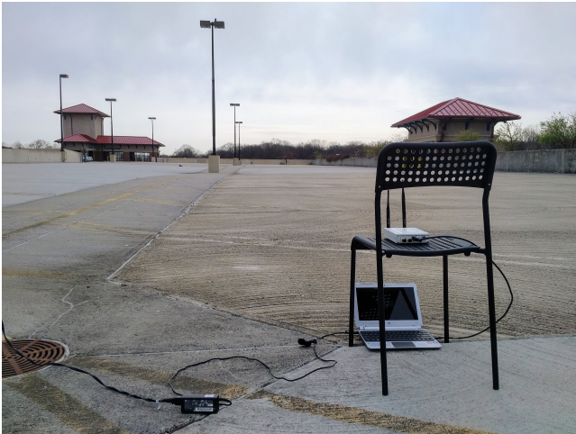
Figure 8: The test area that was used for distance measurements. Sender and receiver are 100 meters apart.
