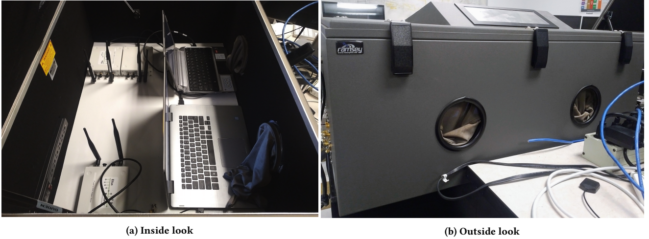
Figure 5: Faraday Cage setup
