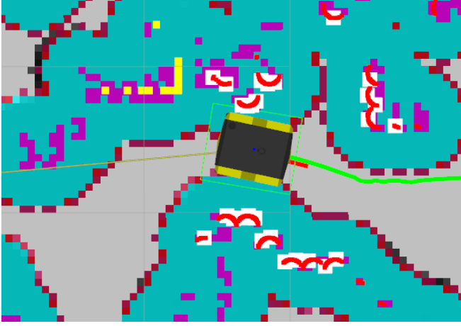
Fig. 5: Rviz visualization of obstacles in the MPC. White squares: obstacle coordinates sampled from raw LiDAR scan. Yellow squares: blind spot obstacle coordinates obtained from local_costmap .
