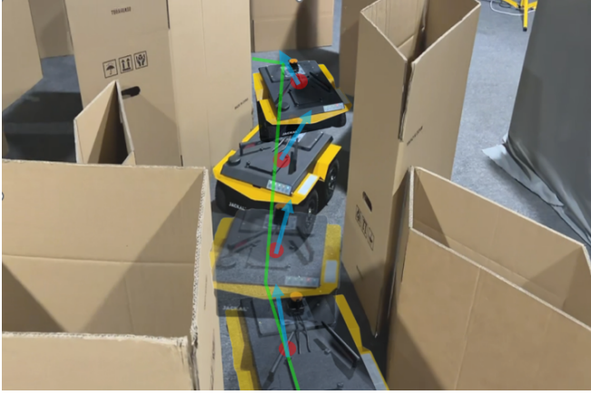
Fig. 4: Physical experiment of VFH*-based local obstacle avoidance. The green line represents the global path, and the blue arrow indicates the local obstacle avoidance direction selected by VFH*.
