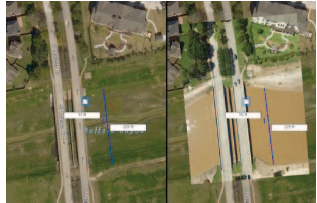
Figure 2 Pre-flood view of a base map (left) of S Mason Rd crossing Buffalo Bayou in Katy, TX and post-flood view with superimposed SUAS image (right). Pre- and post-flood water width measurements are shown on both.
