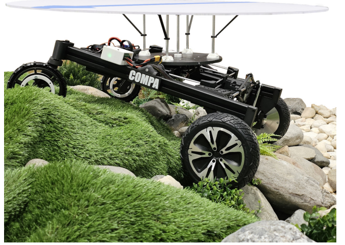
Fig. 1: COMP A demonstrating the ability to keep the turret horizontal (white plate) and directed (blue arrow), independent of the base pose, during holonomic off-road navigation.
