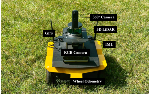
Fig. 2: Robot Setup: We use a Clearpath Jackal for dataset collection, which is equipped with various sensors, including 3D LiDAR, RGB camera, 360° camera, IMU, and GPS. It is capable of traversing diverse terrains, including pedestrian roads, roadways, off-road areas, ramps, and woods.
