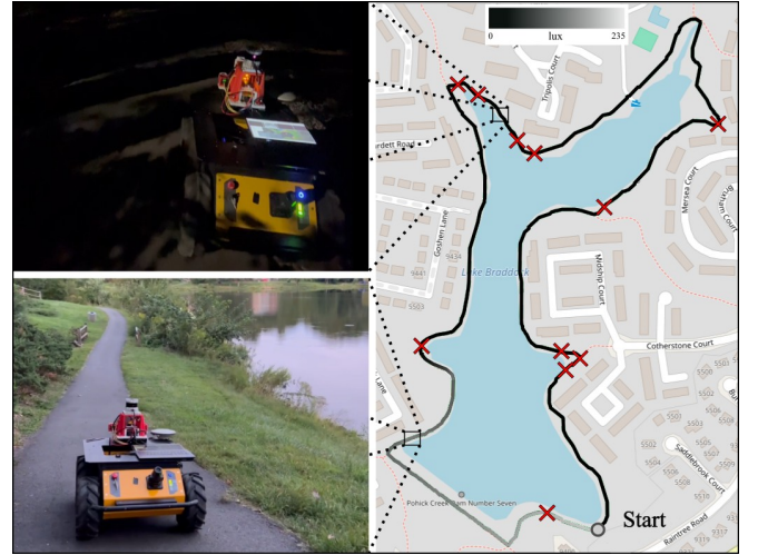
Fig. 8: Autonomous Navigation around a 3.6 km Trail with a BC model and Thermal Input: Lighting conditions drops from 255 lx at the beginning (light gray on the path, lower right) to 0 lx (black, upper left). 11 interventions (red crosses) are necessary to correct the robot when going off-course.
