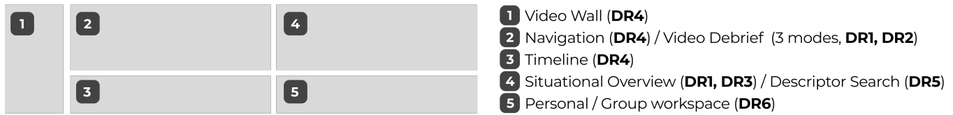
Figure 3: MRVS interface layout and corresponding design requirements.
