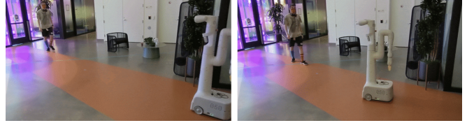
Fig. 1. Frontal approach scenario: human and robot interact by moving along a straight trajectory in opposite directions (left). The robot yields early on to not block the human from walking along their path (right).
