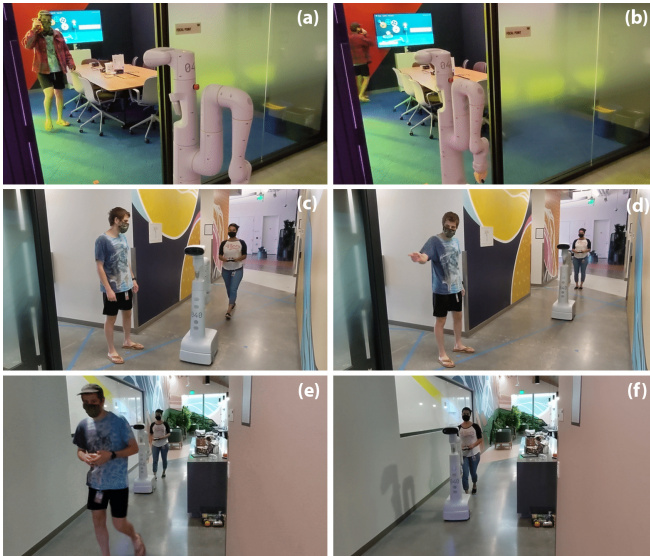
Fig. 4. Examples of the social scenarios: narrow doorway (a, b), intersection gesture (c, d), and intersection wait (e, f). Each scenario is defined by enacting the social interaction with a human and a robot that is manually controlled by a human operator.
