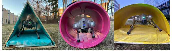
Fig. 1: SQUID is deployed in real-world tunnel environments, demonstrating the adaptability and robustness of the proposed approach. The quadrupedal robot relies on limited visual perception to navigate confined spaces, successfully traversing narrow passages and uneven terrain.
