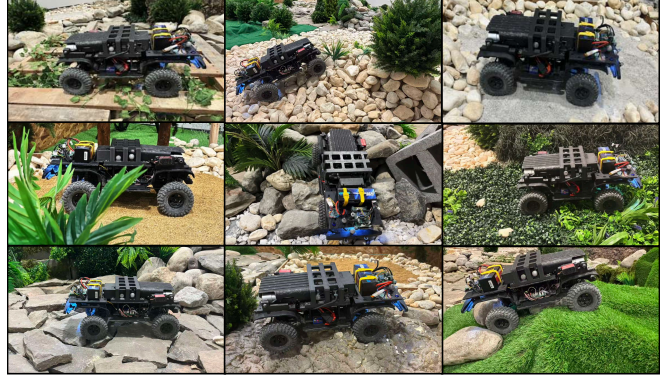
Fig. 1: Facing a variety of constantly changing elevation and semantics on vertically challenging, off-road terrain, autonomous mobile robots need to quickly adapt their terrain understanding through online kinodynamics adaptation to achieve safe and efficient navigation.
