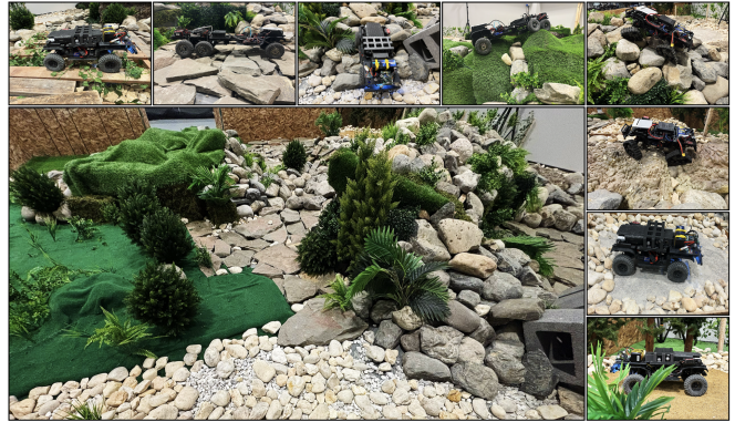
Fig. 1. Verti-Arena comprises a variety of off-road terrain, includes different geometries and semantics, and is equipped with a motion capture system, to facilitate off-road autonomy research.
