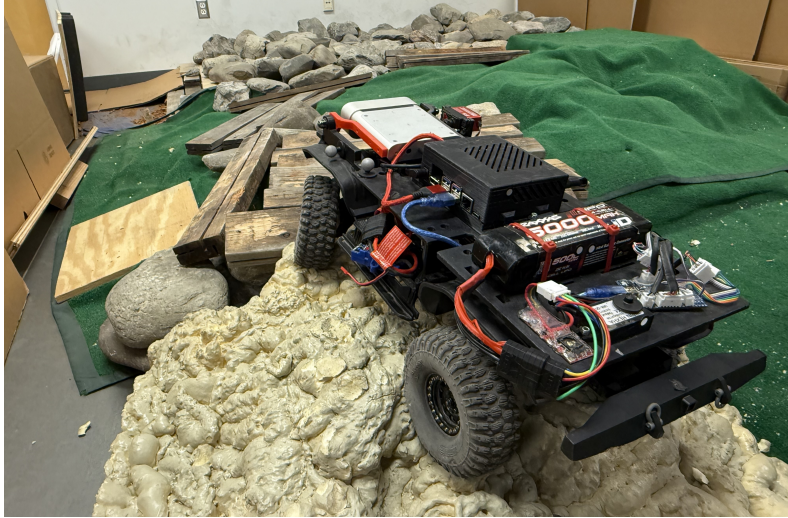
Figure 7: Unseen Test Environments with Rocks/Boulders, Wooden Planks, AstroTurf, and Expanding Foam.
