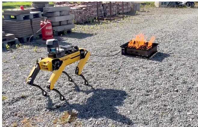
Fig. 1: Experimental setup with the Boston Dynamics Spot robot approaching a controlled fire generated by a propane-based fire training device. The robot is equipped with depth and thermal sensors to perceive the environment and construct a thermal radiation field for fire-aware navigation.
