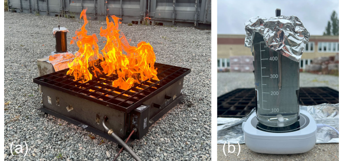
Fig. 10: To estimate the thermal radiation, we performed a calorimetry experiment. We measured the time it takes to increase the temperature of 500ml of water 45cm away from the center of the fire.
