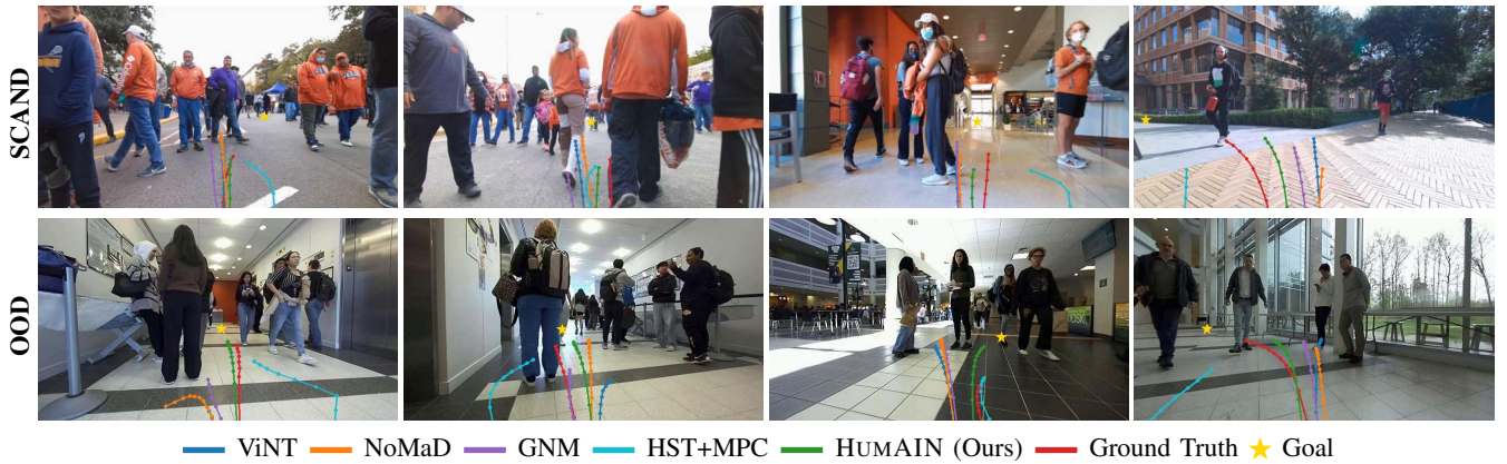
Fig. 4: Qualitative Results: Generated trajectories are projected onto the robot ego-centric view images using all the methods, ViNT [37] in blue, NoMaD [38] in orange, GNM [44] in purple, HST [11] with MPC [45] in cyan, HUMAIN in green, and the ground truth trajectory in red. The target goal is marked with a yellow star. The top row shows SCAND test dataset results, and the bottom row shows the results on the out-of-distribution dataset that we collected.
