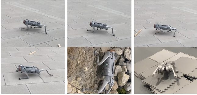
Fig. 5: Disturbance recovery cases on diverse terrains (zero-shot Go1): The above cases demonstrates that our policy experiences a bump/trip or deviate laterally, and re-stabilizes to its normal gait within few seconds. Above examples demonstrate that TransCurriculum-trained policy remains functional without any additional finetuning under disturbances or terrain irregularities (See accompanying video).
